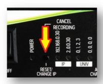
When in reset mode, it is possible to easily choose between the following IP addresses, by pressing the "RESET/CHANGE IP" button:
